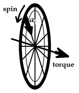
2-D spinning wheel creates constant point-by-point centripetal acceleration inward as well as torque perpendicular to the plane of the wheel
